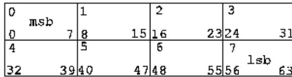
Figure 1-3. Bit and byte numbering in doublewords
